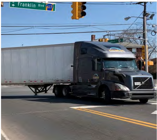
Heavy vehicles encroaching onto Somerset Street left turn lane onto Franklin Boulevard
